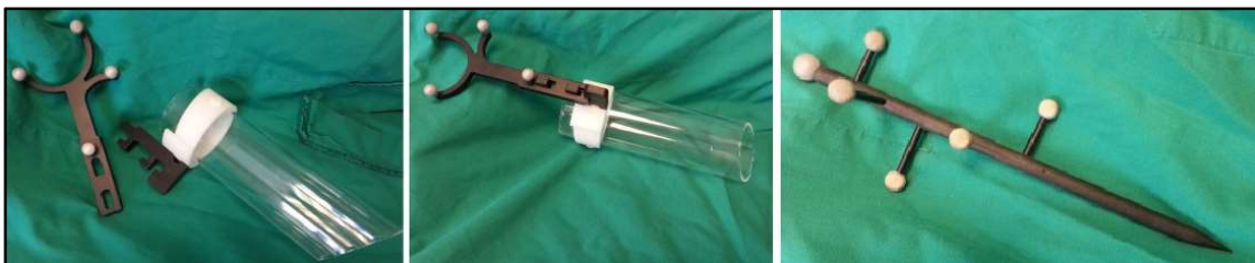
Figure 14. Surgical Tools with Integrated IR-Markers [13]
