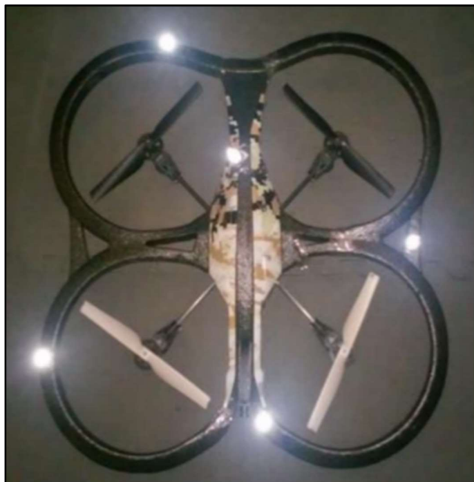
Figure 54. Autonomous Drone Equipped with Reflective Motion Capture Markers [37]
