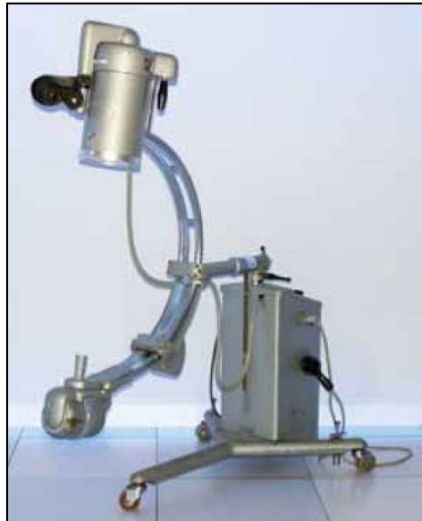
Figure 7. The BV 20 First Surgical C-Arm [6]
