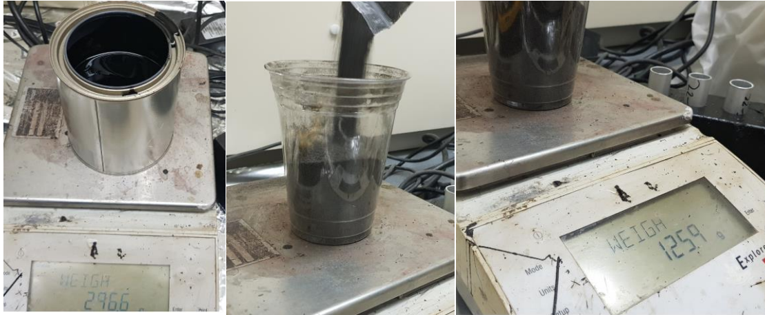
Figure 10. Determination of the Required RAR Weight for Virgin Binder Modification.
