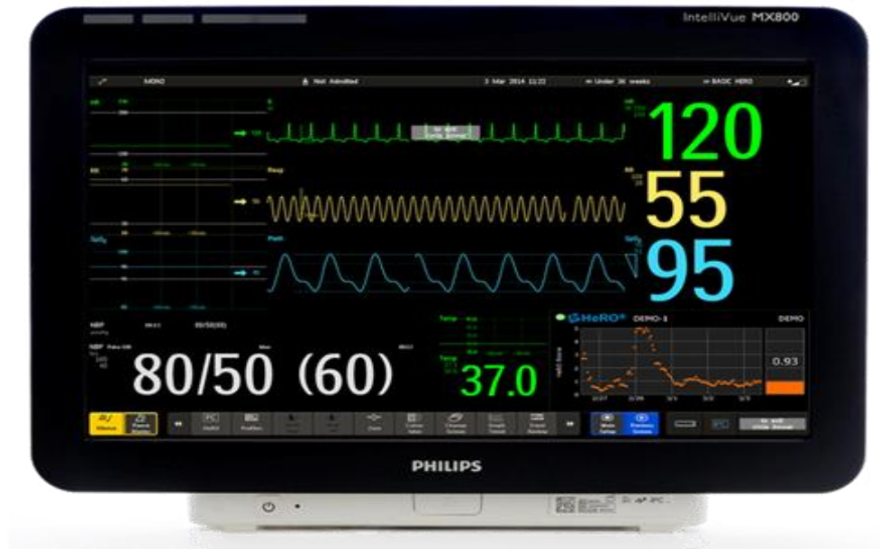
Figure 2.3 Infants monitor displaying HR, RR, SpO2%, pulse and temperature [23]
