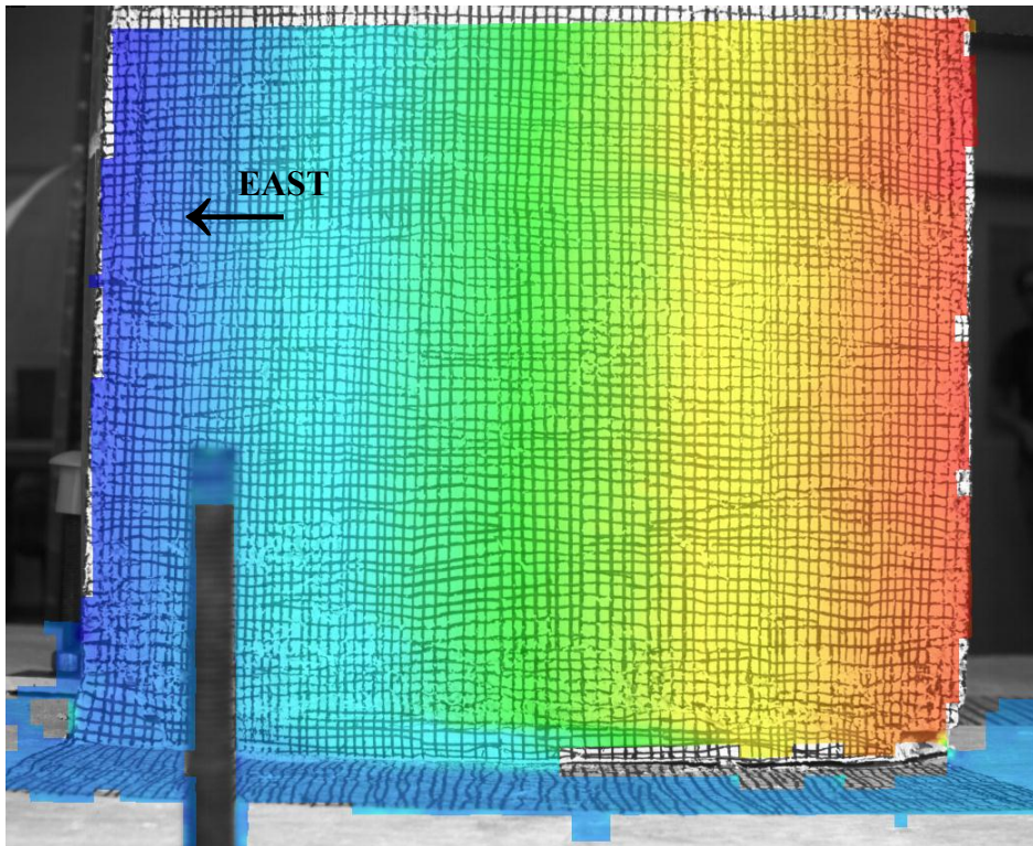
Figure 3.38: FOV Compression Pier Base (Looking South): System 3 (2D)
