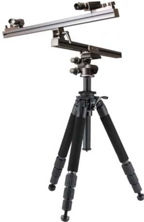
Figure 2.8: 3D-DIC Physical Setup
