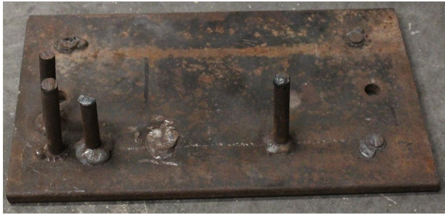
Figure 5.2: Steel Jig Used to Bend Rebar
