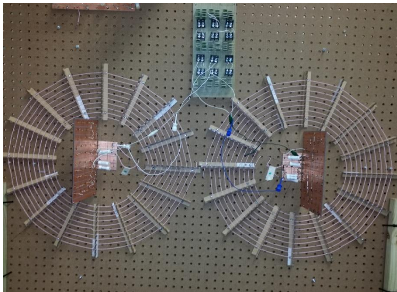
Fig. 4.6 Fabricated resonators L_5 (left) and L_4 (right). The circuit board between the two coils is a load block consisting of nine clusters of 50\Omega noninductive power resistors which could be combined to form various resistance values. At the center of each coil are found fixed capacitors and sheet capacitors for precise resonator tuning.
