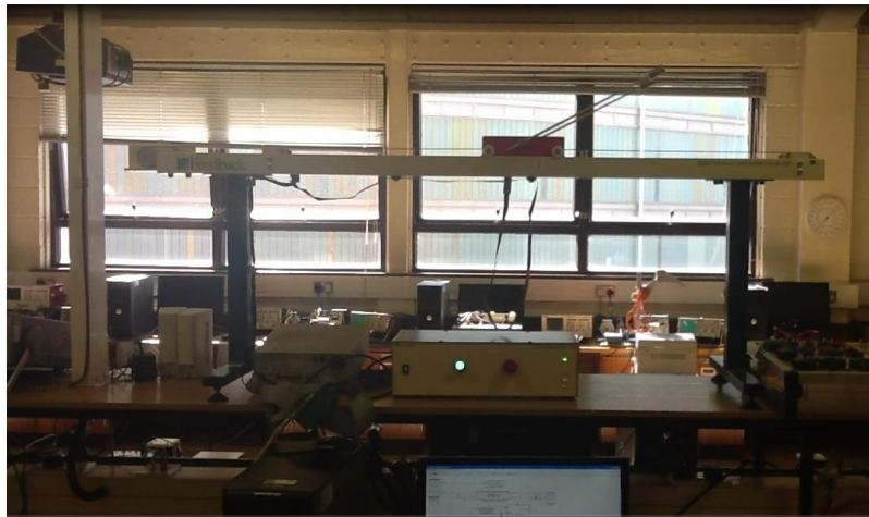
Figure 9. Pendulum in swing-up mode by swinging controller
