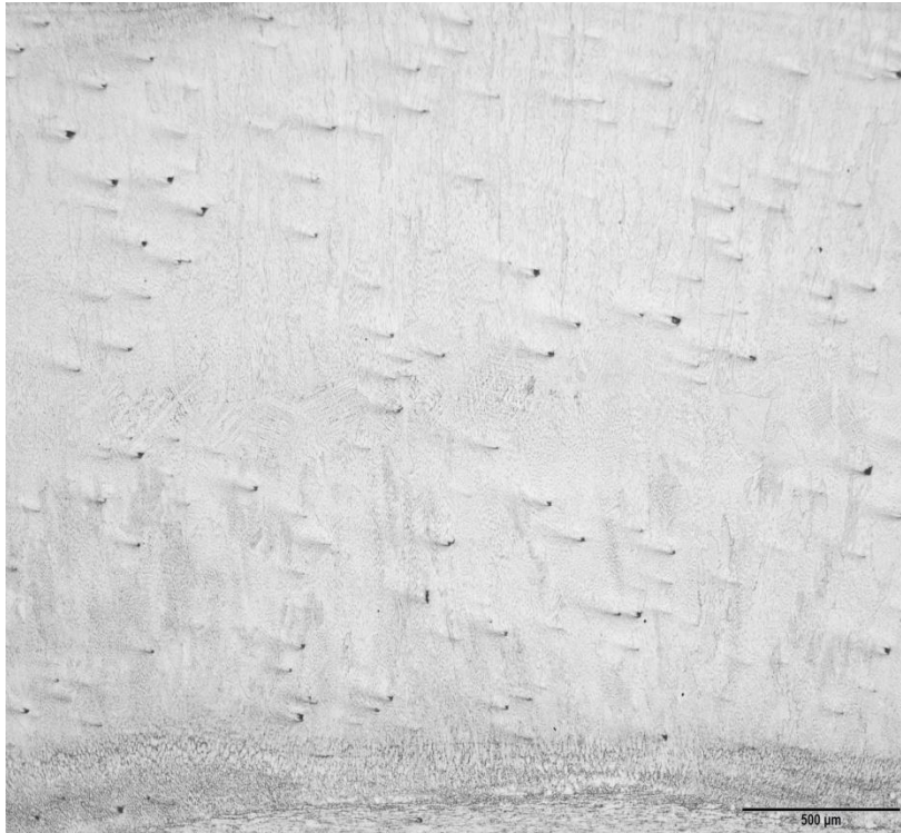
Figure 5. Weld structure of optimized model
