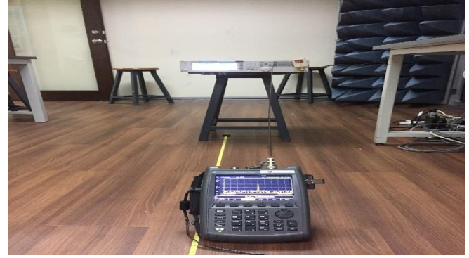
Figure 7: Experimental setup adopted to evaluate the signal strength of the antenna in term of the range distance.
