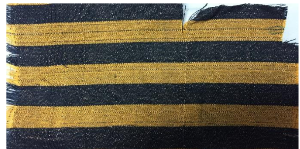
Figure 4: Photograph of E-textile that consists of copper thread and polyester thread.
