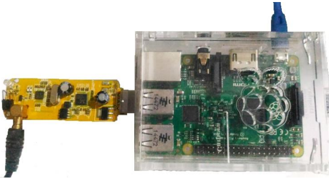
Figure 4: Hardware of the WebSDR
