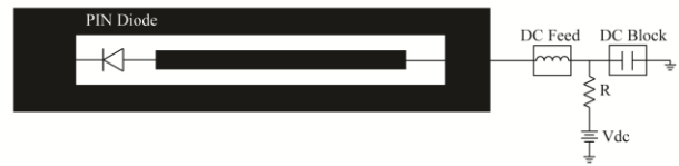
Figure 6: Proposed tunable U-shape DMS
