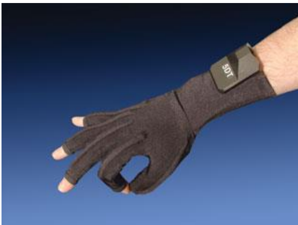
Figure 1: 5DT data glove for hand motion tracking
