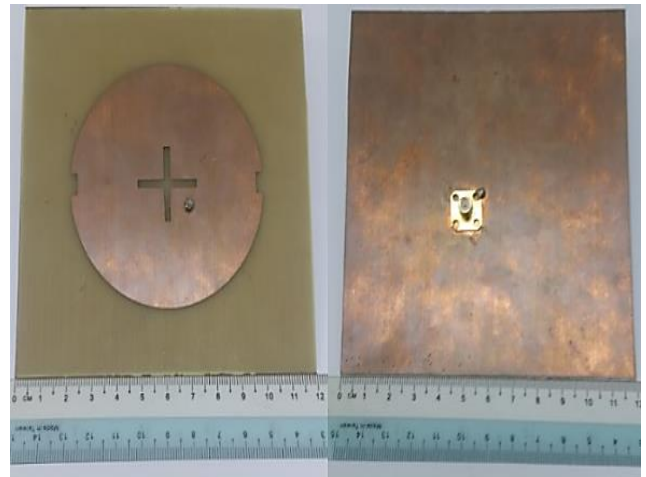
Figure 2: Fabricated Microstrip Antenna
