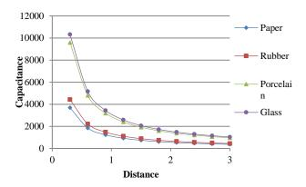
Figure 7: Graph of capacitance over distances for different materials
