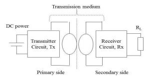
Figure 1: General circuit configuration for Wireless Power Transfer system
