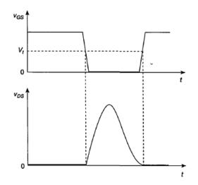
Figure 5: Waveforms of gate-to-source voltage ( $V_{GS}$ ) and drain-to-source voltage ( $V_{DS}$ ) in Class E qero-voltage-switching power amplifier
