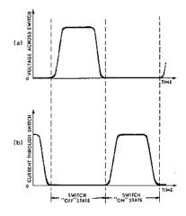
Figure 2: Optimum waveforms in Class E circuit arranged for maximum power efficiency [8]
