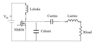
Figure 4: Basic Class-E circuit configuration [10]
