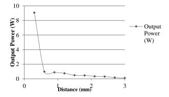
Figure 9: Graph of output power for increasing distance
