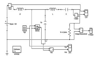
Figure 6: Design of Class E power amplifier used for the simulation work
