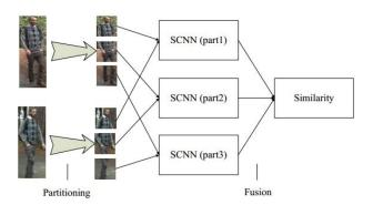
Figure 7: Flowchart of Siamese Convolution Neural Network [38].
