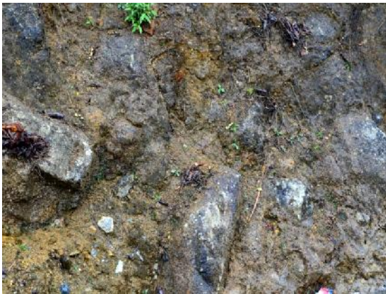
Figure 9. Colluvial deposits along the road from Tam Duong to Lai Chau (Photo in January 2015)
