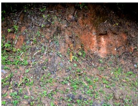
Figure 10. Colluvial deposit along the road from Dien Bien to Tay Trang (Photo in January 2015)
