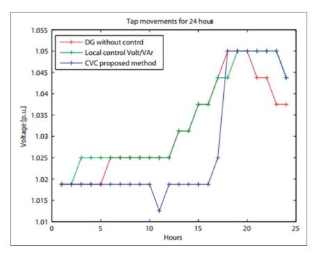
Figure 6. Result of OLTC tap movements for 24 hours, with proposed CVC and the two comparative scenarios
