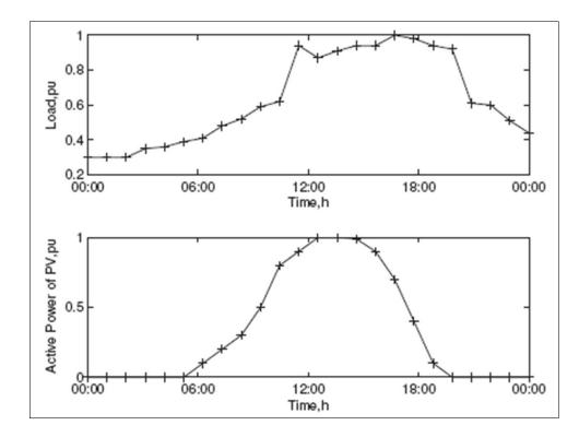
Figure 2. Daily system load and DG power production profiles
