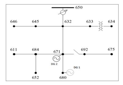
Figure 3. Diagram of the IEEE 13 Node test Feeders and the two PV DG connections
