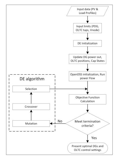
Figure 1. Flow chart of proposed DE-based CVC algorithm
