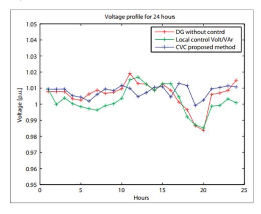
Figure 5. Daily voltage profile comparison at bus 680, from phase A - with the proposed DE-based CVC method and the two comparative scenarios
