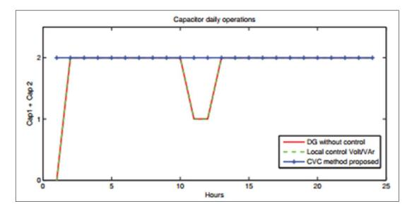
Figure 7. Capacitors status for 24 hours with proposed CVC
