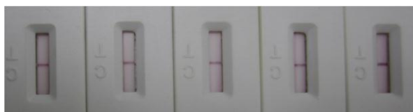
Figure 6. Conjugation of different amounts of rabbit anti-rotavirus IgG with gold nanoparticles to generate the conjugate pad.
