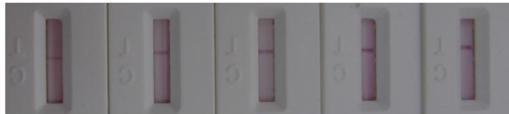
Figure 7. Immobilization of different amounts of guinea pig anti-rotavirus IgG on the nitrocellulose membrane as T-line of LFA strip.
