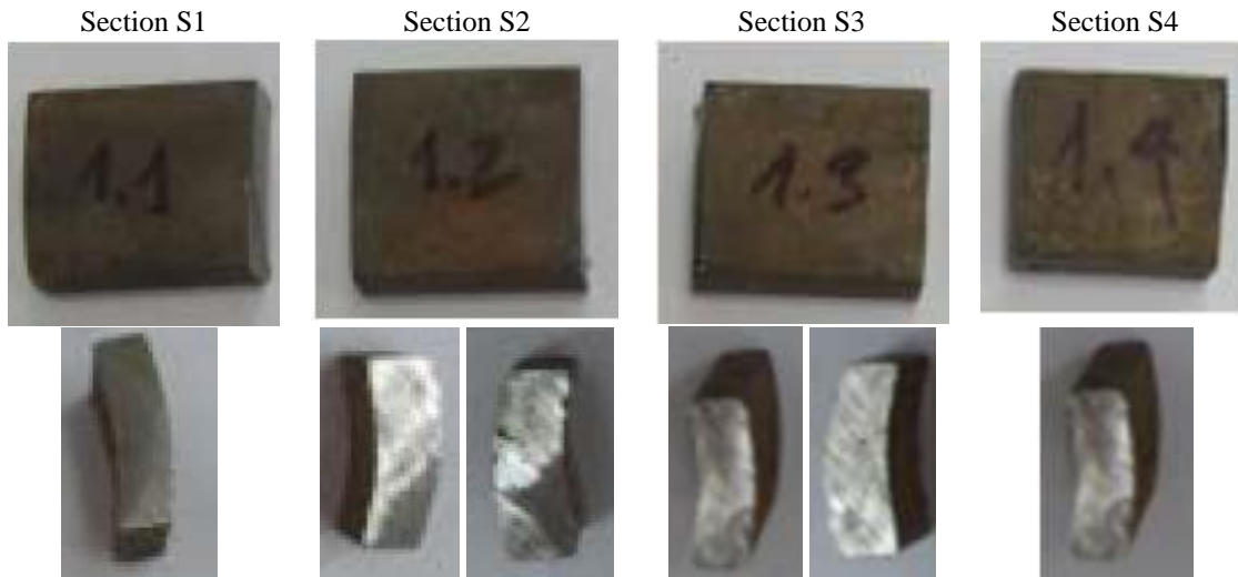
Figure 6. Visual test of surface of sections for testing samples in HIC test.
