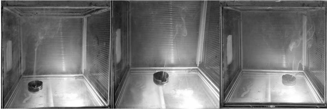
Fig. 10. The experimental illustration of contaminant spreading in a natural convection in a box
