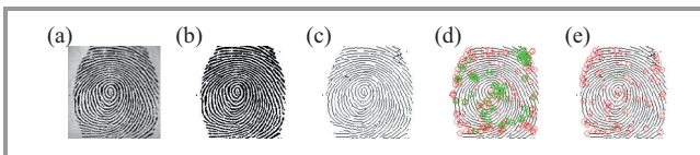
Fig. 4. The proposed fingerprint authentication systems implemented on the LG Nexus 5: (a) the original fingerprint image, (b) the binarized fingerprint image, (c) the thinning fingerprint image, (d) detected minutiae, (e) the minutiae (end points and bifurcations) extracted after checking its distance.
