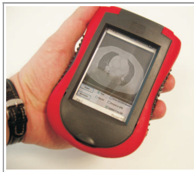
Fig. 2. Current portable devices come in compact rugged cases and feature build-in wireless LAN connectivity.
