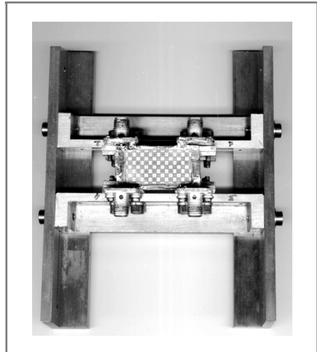
Fig. 8. Photography of fabricated coupler with SMA connectors prepared for measuring.
