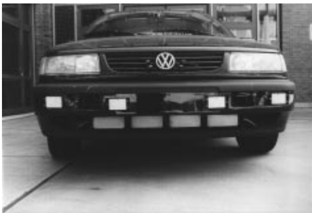
Fig. 4. Experimental vehicle equipped with a short range radar sensor network.
