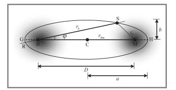
Fig. 2. Eccentro-scattering model for picocells and microcells.
