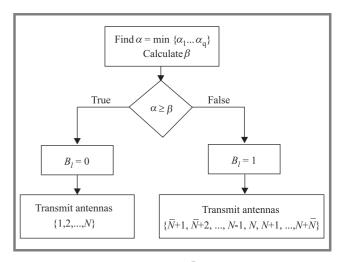
Fig. 5. The flow chart of the  $(N + \overline{N}, N; K)$  AST/DSTBC.
