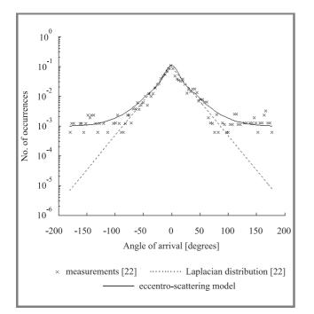
*Fig.* 7. Comparison of the pdf of AoA for eccentro-scattering model (a = 36 m, D = 64 m, and  $\sigma_m = \sigma_b = 18$ ), Laplacian distribution ( $\sigma = 25.5^{\circ}$ ) [22], and measurements [22].
