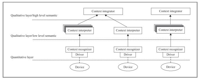
Fig. 9. Context detection using sensors.
