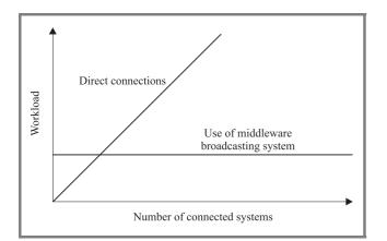
Fig. 2. Workload produced by connected systems.
