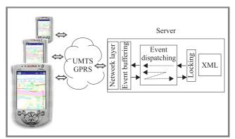
Fig. 6. Collaborative SVG system architecture.
