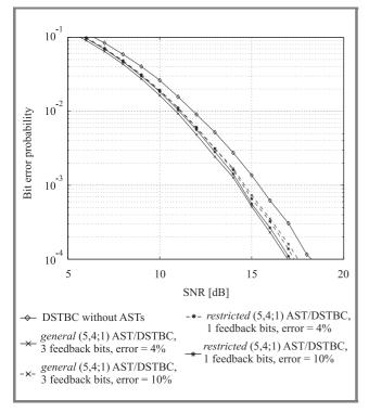
*Fig. 10.* Square, order-4, unitary DSTBC with the *general* (5,4;1) AST/DSTBC and the *restricted* (5,4;1) AST/DSTBC schemes.
