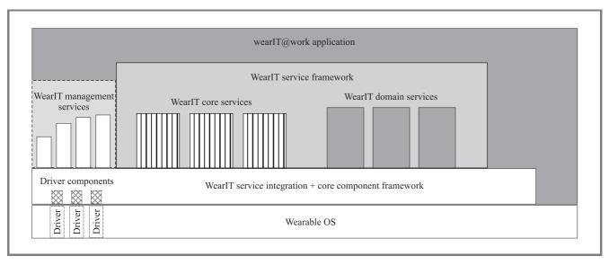
Fig. 7. General structure of the software framework.
