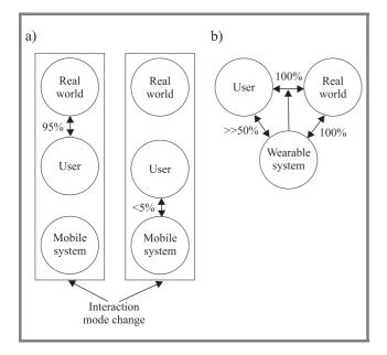
*Fig. 2.* Interaction between the user, the system and the environment in a conventional mobile system (a) and a wearable system (b).
