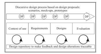
Fig. 3. Generic ISO 13407 compliant UCD process model.
