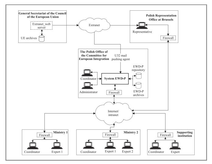
Fig. 1. The EWD-P system architecture.
