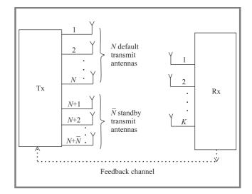
Fig. 4. The diagram of the  $(N + \overline{N}, N; K)$  AST/DSTBC.
