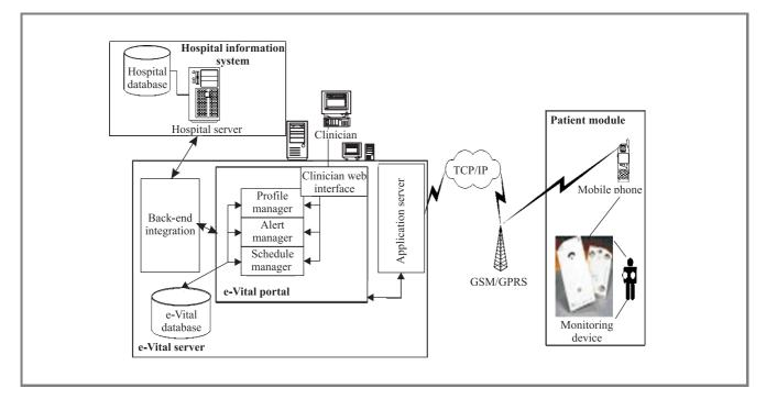
Fig. 4. The e-Vital system architecture.
