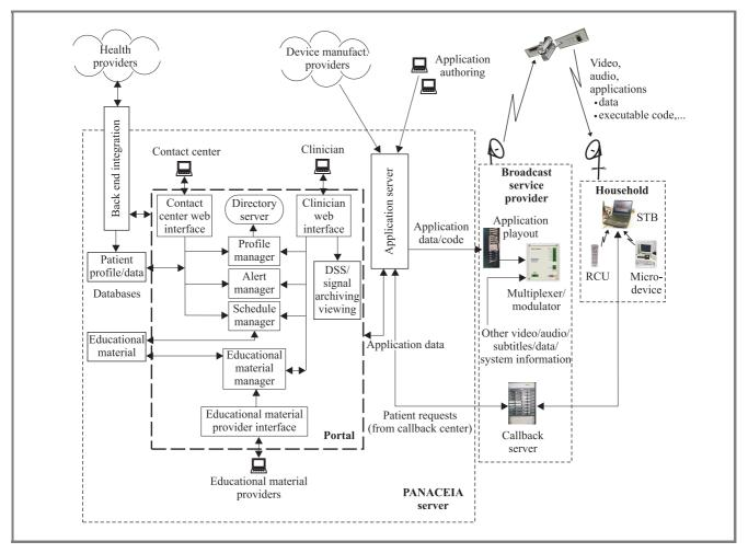
Fig. 3. The PANACEIA-iTV system architecture.
