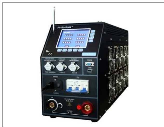
Fig. 2. Battery discharger with nominal current of 120 A.
