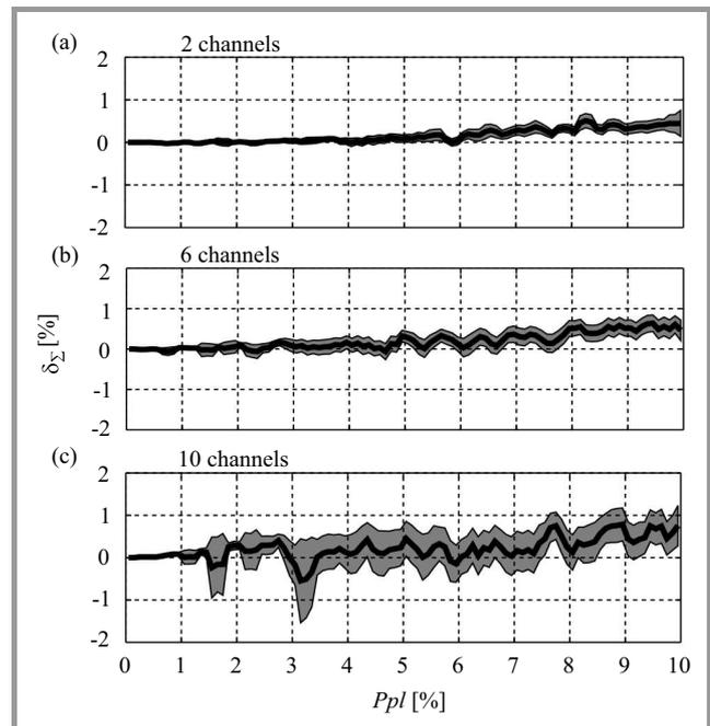
**Fig. 5.** Relationship between the burst ratio calculation error  $\delta_{\Sigma}$  and the packet loss rate  $Ppl$  of the whole transmission. The solid line represents mean relative error while the gray areas present the 95% confidence intervals of the mean. The figures were created with a packet loss range of 0–10%. The subplots presents results for simulations of two, six and ten intermediate channels.
