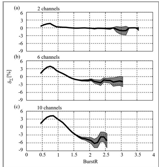
**Fig. 7.** Dependency of the burst ratio calculation error  $\delta_{\Sigma}$  on the  $BurstR$  value of the complete transmission. The solid lines represent mean relative error while the gray areas present the 95% confidence intervals of the mean. The subplots presents results for simulations of two, six and ten intermediate channels.
