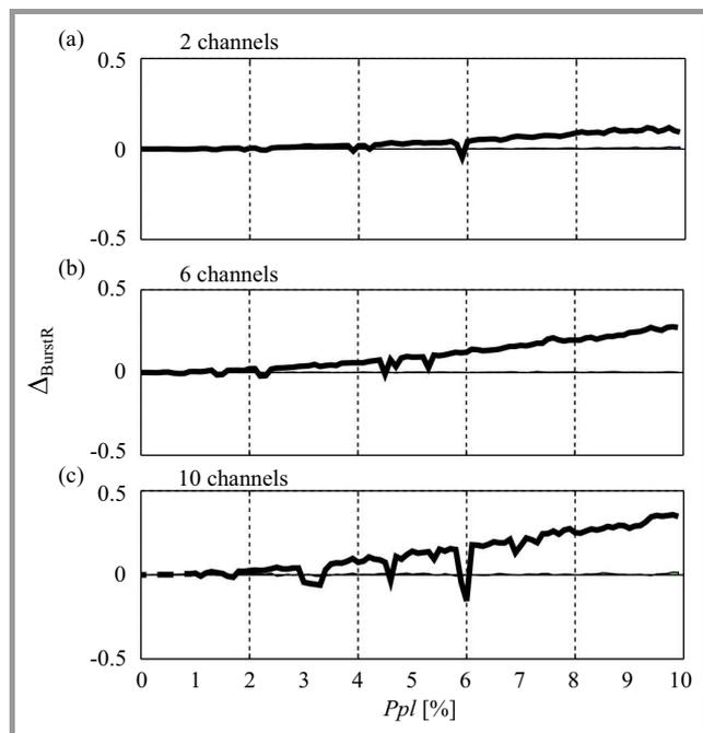
**Fig. 8.** Difference  $\Delta_{BurstR}$  between the calculation errors of the regular equation  $\delta_\Sigma$  and the simplified equation  $\delta'_\Sigma$  in the domain of packet loss  $Ppl$  of the whole transmission. The solid lines represent the difference between mean relative errors while the gray areas represent the difference between the 95% confidence intervals. The subplots presents results for simulations of two, six and ten intermediate channels.
