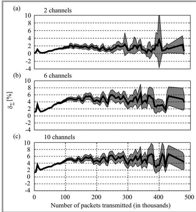
**Fig. 6.** Relationship between the burst ratio calculation error  $\delta_{\Sigma}$  and the number of transmitted packets. The solid lines represent mean relative error while the gray areas present the 95% confidence intervals of the mean. The subplots presents results for simulations of two, six and ten intermediate channels.
