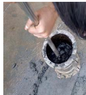
Fig 3.4.2 A) PLACING OF CONCRETE IN MOULD Fig 3.4.2 B) SPLIT TENSILE STRENGTH TEST
