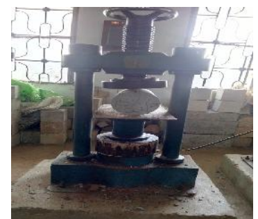
Fig 3.4.2 A) PLACING OF CONCRETE IN MOULD Fig 3.4.2 B) SPLIT TENSILE STRENGTH TEST
