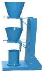
Fig 3.1.2 compaction factor apparatus
