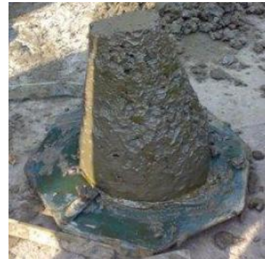
Fig 3.1.1 Slump Test Reporting of Results:
