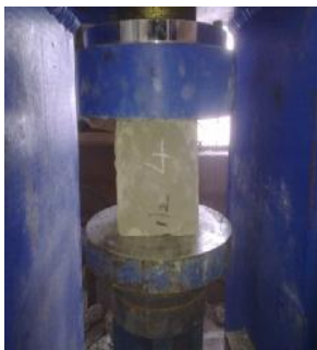
Fig 3.4.1 E) Before and after application of load by Compression testing machine
