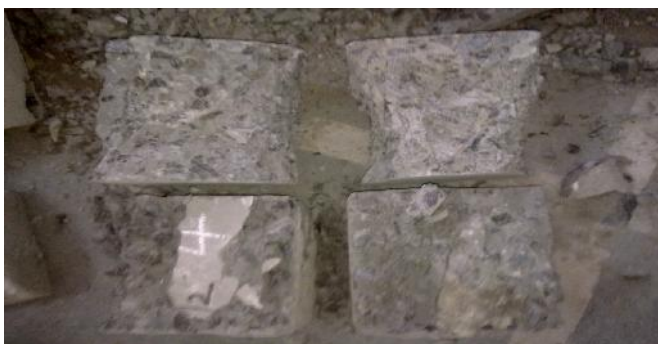
Fig 3.4.1 F) Specimen after Testing in Compression testing machine
