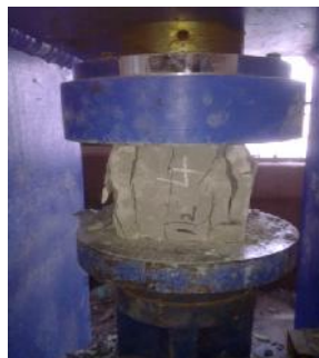
Fig 3.4.1 E) Before and after application of load by Compression testing machine
