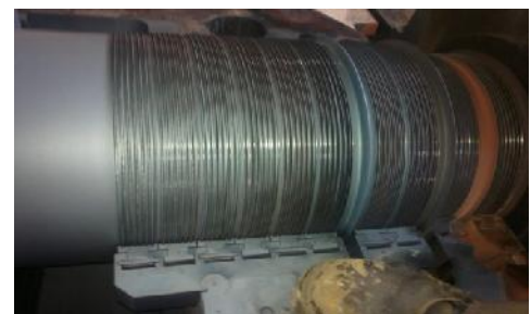
Fig. 6. Arrangement of glands to the turbine rotor
