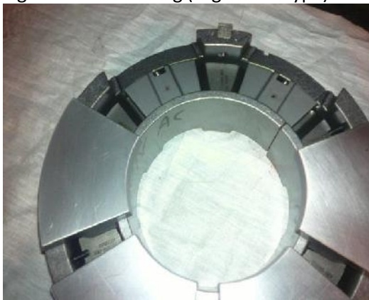
Fig. 3. thrust bearing (tilting type)
