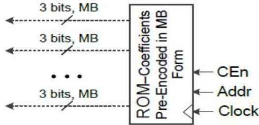
Fig.4 the ROM of Pre-Encoded multipliers with standard coefficients in MB form.
