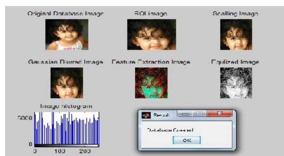
Fig. 2 Feature Extraction of Database Image Smoothing process is used and by adding Gaussian noise to the image to get Gaussian blurred image . By ROI and Scalling to process cropping the image and resizing the image can be done. Using Local Binary Pattern by size of width and height of image the Database image feature is extracted.
