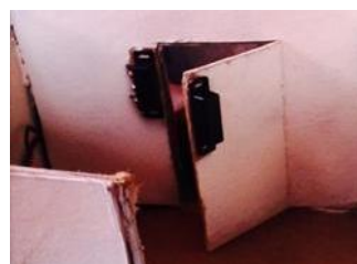
Fig. 6 Entry detection using Reed Switch
