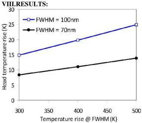
The result shows head temperature varies with media temperature.Head temperature increases linearly with increased mediatemperature, and it rises faster for larger spot.
