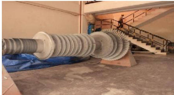
Fig.5 32MW Turbine rotor
