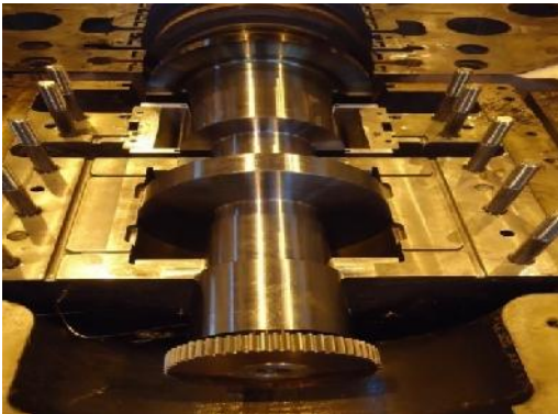
Fig. 2 Turbine base plate with front bearing pedestal
