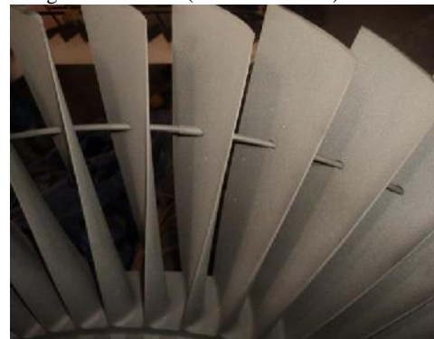
Fig. 4LP Blades (lashing wired blades)
