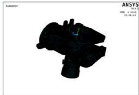
Fig 7.3 Meshed shape of Carburetor in ANSYS
