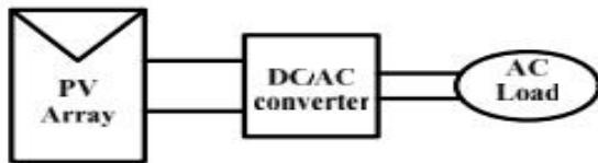
Fig. 11: Block diagram representation of Photovoltaic system
