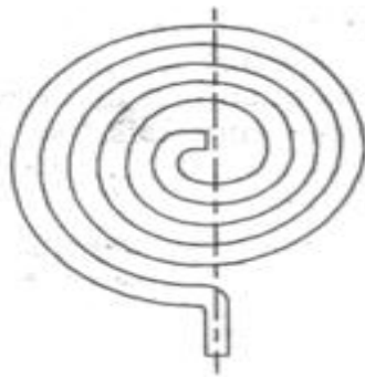
(b) Spiral torsion spring.
