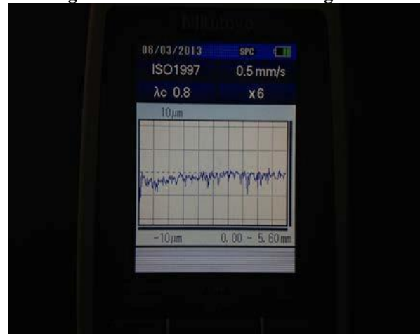
Fig-3: Surface Roughness Illustration
