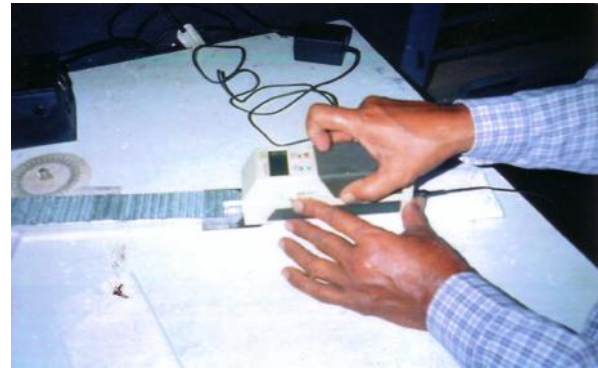
Fig-2 Measurement of surface roughness
