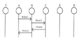
TWOACK detects mischievous links by acknowledging every data packet transmitted over every three successive nodes along the path from the source to the destination. Upon recovery of a packet each node along the route is necessary to send back an acknowledgment packet to the node that is two hops away from it down the route. TWOACK is required to work on routing protocols such as Dynamic Source Routing (DSR).
