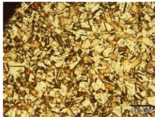
Fig-21 , Microstructure after final pillgaring outside tube
