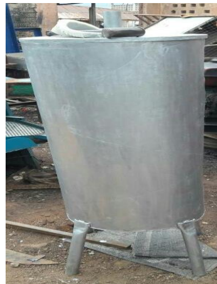
Plate 3: The sludge dewatering filter
