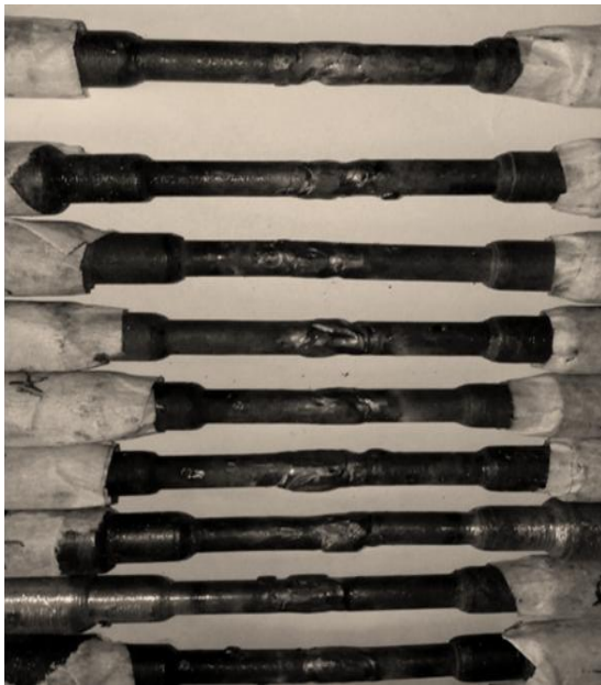
Fig. 1: Post heat treated welded samples
