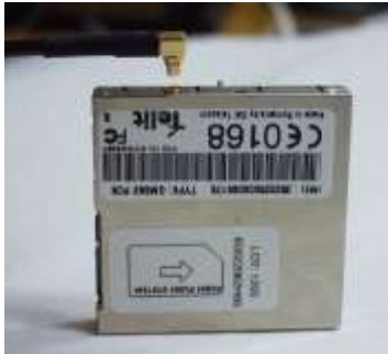
Fig. 3: Telit Module showing connection of GSM Antenna
