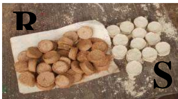
Plate 4: Rice Husk Briquette (RHB) and Saw-dust briquette (SB) produced from the developed machine
