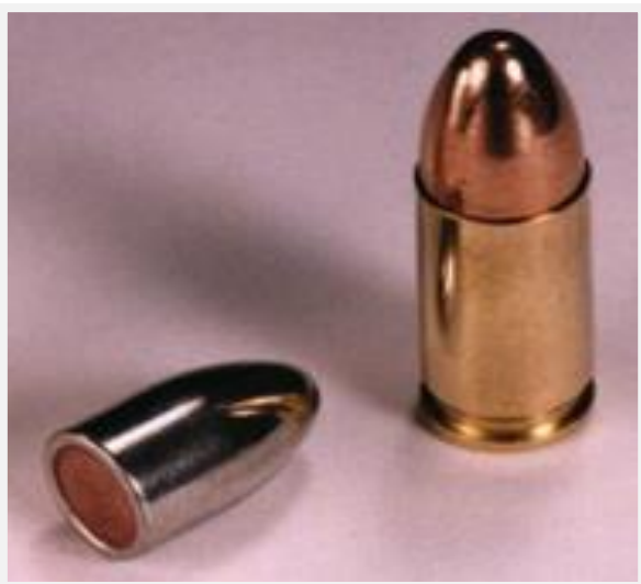
Plate 1. 9x19mm ammunition (ball and the assembled bullet) used for the ballistic experiment
