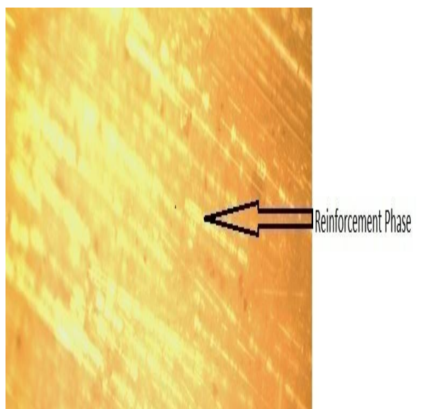
Plate 3. Micrograph showing the compatibility of the constituent materials in the fabricated PMC (X200)
