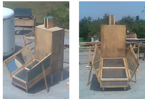
Fig. 2. Semi-active solar dryer when mirrors were attached
