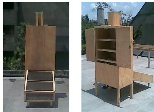
Fig. 1. Front and Rear view photographs of the semi active solar dryer
