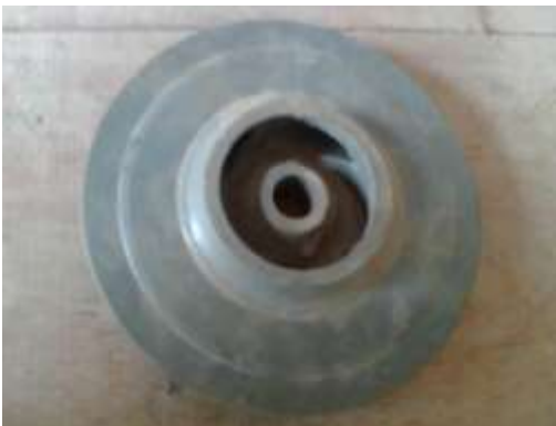
Fig. 7: Finished cast impeller
