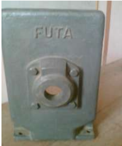
Fig. 5: Finished cast pump housing front view.
