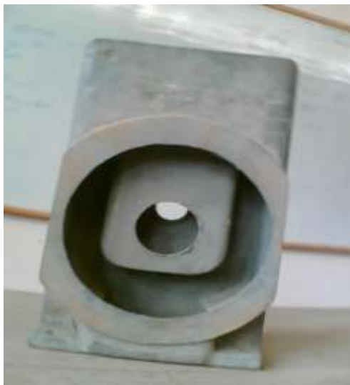
Fig. 6: Finished cast pump housing back view
