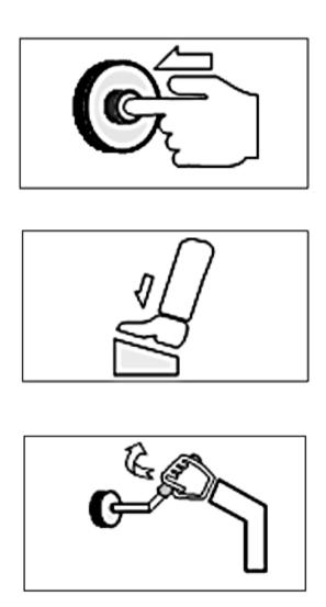
**Figure 3.1** Uncoloured pictograms for required actions in emergency situations: push a button, step on a pedal, and turn a handle
