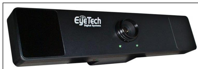
**Figure 3.5** EyeTech TM3 non-intrusive eye tracker
