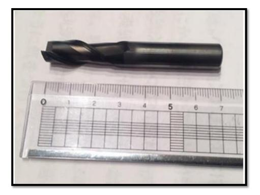
Figure 2.7 CVD-diamond coated end-milling tools with the film thickness of 15 μm
